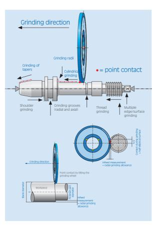
The standard QUICKPOINT grinding operations are shoulders, tapers, chamfers and grooves. Thread grinding and multiple edge and face grinding can be additionally integrated.
