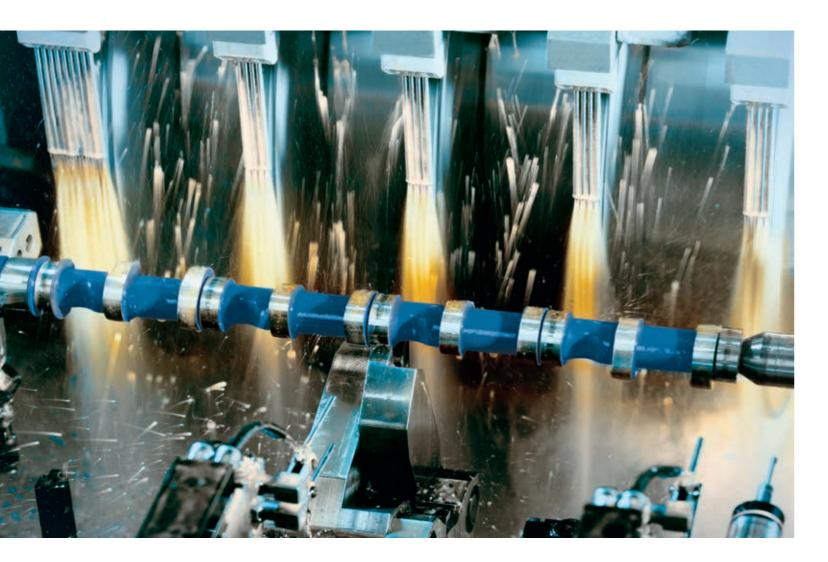
The JUCENTER CBN high-speed grinding machine combines mutually complementary grinding possibilities under one hood. Instead of lining up individual grinding machines for different grinding tasks, both grinding processes take place in two separate clamping set-ups on one machine. The result: highly efficient grinding – all with top precision.
