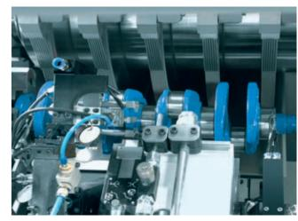
Grinding station 1: Circular grinding of main bearings with grinding wheel set
