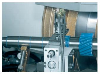
Grinding of diameters on transmission parts with sets of grinding wheels
