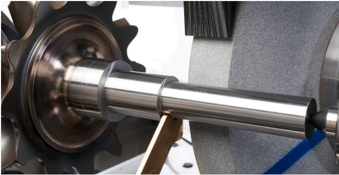
Diameter and face grinding on turbocharger shafts
